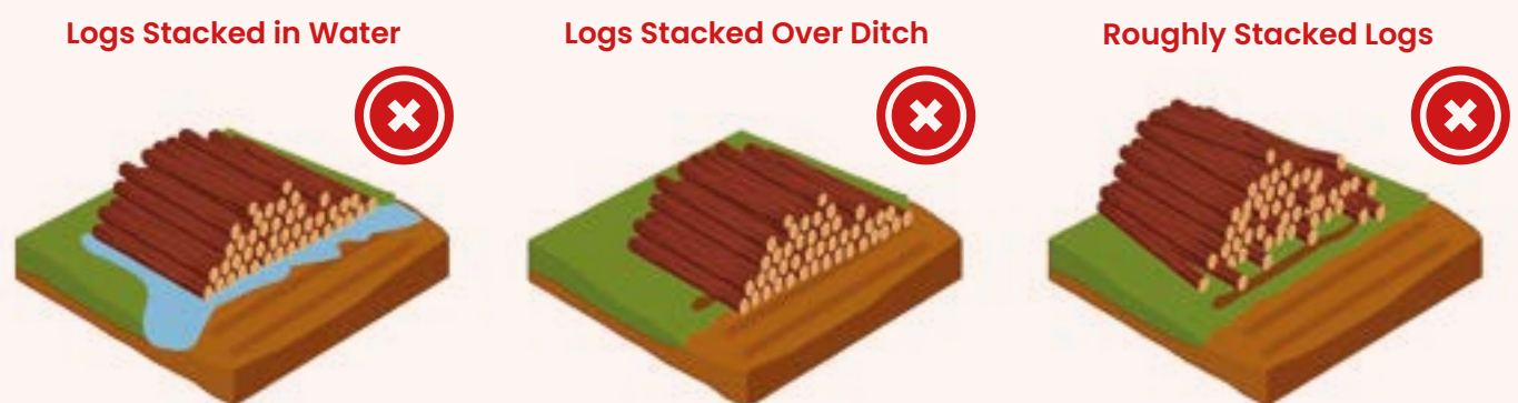
Figure 2: Advice for stacking timber in the forest.
