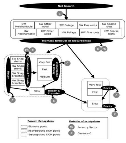
Figure 1: A schematic summary of how annual processes and C transfers between pools are simulated in CFS-CBM model (taken directly from Kurz et al., 200911). Note that forestry sector (FS) products (i.e. harvests) are allocated to the HWP model (Figure 1).
