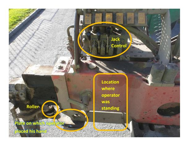
When fully retracted, the roller sits into a hook to securelly lock the jacks for travel. Hydraulic force from the retracting extendible jack arm powers the roller into position.
