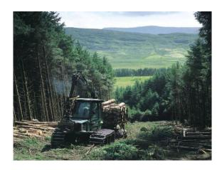
The logs are systematically stacked for open air drying down to the required moisture contents specific to each customers boiler requirements. The key to ensuring quality wood chip at the correct moisture content is to manage stock rotation and replenishment and to ensure suitable air flow through the stacks.
